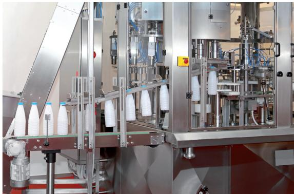
Lubrication of crimpers and suspension conveyors for PET bottles in the food industry
