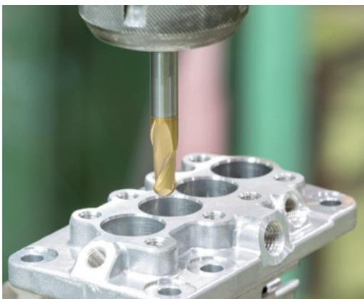
Center point drilling on light aluminium-silicon alloys, 4000 Series (Aluminum-Silicon Wrought Alloy)
