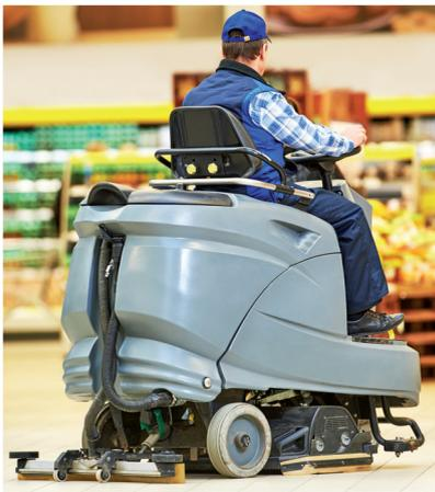
Cleaning of floors with walk behind scrubbers or rider scrubbers, equipped with water flow control.
