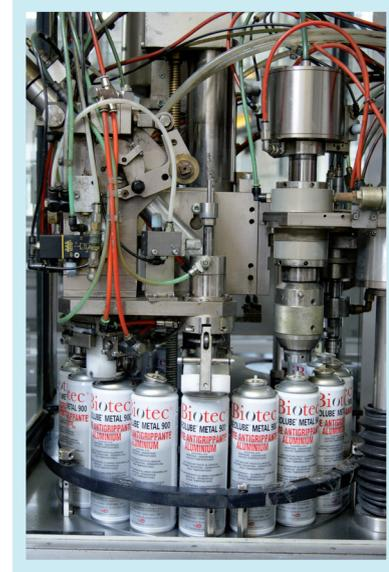
iBiotec is equipped with 3 fully automated filling lines with a combined capacity of 60 aerosol containers per minute per machine.
